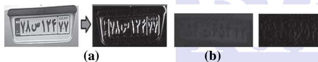
Figure 2.1: Results of applying the Sobel edge detector on (a) a clean plate and (b) a dirty plate.
